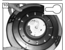
Loosen 4 screws in motor housing then lower metal disk with glass onto fan by aligning 4 key slot holes in metal housing with 4 screws ir fan housing. Tighten the 4 screws securely.
